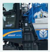
Both fuel and AdBlue tanks can be filled from the ladder for easy access.
